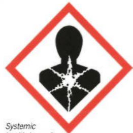
Systemic health hazards
